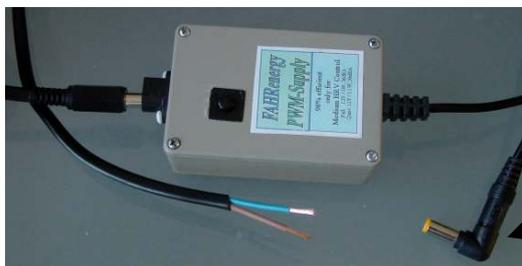
The PWM-Supply is provided with open wires (no plug) due to the lack of a common standard for plugs in caravans.
