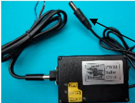
The PWM-Supply is provided with open wires (no plug) due to the lack of a common standard for plugs in caravans.
